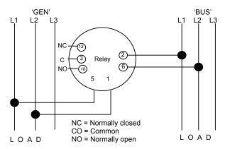
Terminals 3, 10 and 12 are not used on Model 077-14A.
